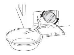
Clean the pump filter and opening.
