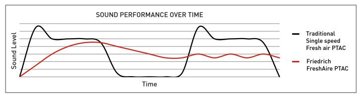
The curves above illustrate the different sound characteristics of a single-speed PTAC (black curve) versus a Friedrich FreshAire® PTAC (red curve).
