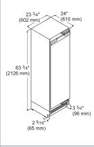
IMPORTANT! Stated minimum height dimensions include when the leveled feet are fully inserted.
