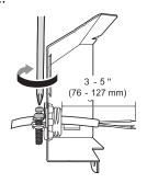
Pull the existing wires through the openings in the junction box. Tighten 2 screws 4 to reassemble the junction box in the appliance.
