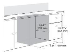
To allow for proper clearance of plumbing and electrical, use the template included with the literature to determine the clearance on the side of the cabinet where the cabinet meets the back wall. Using a 2 1/2" diameter hole saw, drill a hole in the target area as shown on the template.
