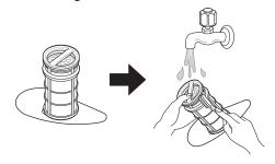
To replace the assembled filters, position the spray arm so the wider vee is toward the front. Fit the filters back into the filter holder and secure them by turning the inner filter clockwise until it clicks into place.
