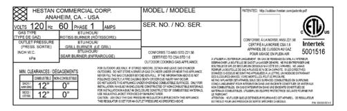
Hestan Grill rating label is located on the underside of the drip pan.
