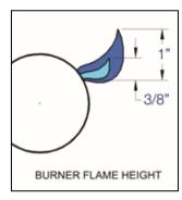
There should be no excessive noise or flame lifting. If any of these conditions exist, remove the burners and check if dirt, debris, spider webs, etc., are blocking the air shutter or burner ports. Proceed with air shutter adjustment if necessary.
