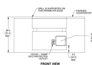
NON-COMBUSTIBLE CONSTRUCTION \_5.25 [13.3] SHOWN 4.0 [10] MIN. 7.63 30.0 [19.4] [76.2] 3.25 \* 8.3 ELECTRICAL BOX LOCATED ON INSIDE REAR WALL OF 23.38 **ENCLOSURE** [59.4] OPTIONAL CABINET AGLP36 [6.4] SIDE VIEW
