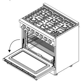
2. Lift up and pull the small levers located on the two hinges all the way back to unlock.
