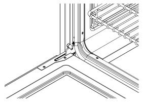
3. Swing the open oven door close until the unlocked levers make contact with the oven frame. The door should be roughly 4" (102 mm) from being completely closed.
