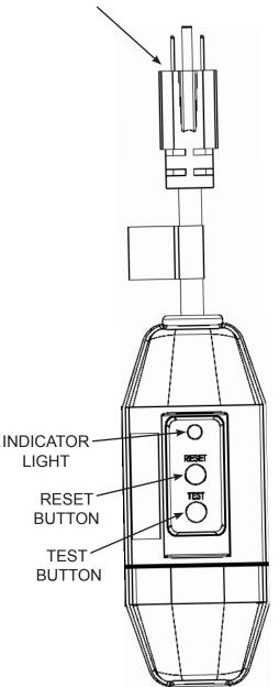
Ground Fault Circuit Interrupter GFCI
