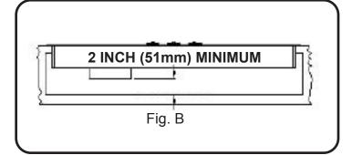
Allow a 2" minimum clearance between the bottom of the metal pan of the cooktop and any combustible surface located below, ie: the upper edge of a drawer installed below the cooktop (see Fig. B). Failure to provide proper clearance and ventilation may result in a fire hazard.
