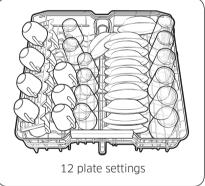
The upper rack is for small plates, mugs, glasses, and plastic items. Make sure the loaded dishes do not interfere with the rotation of the nozzle which is located at the bottom of the upper rack. (Check this by rotating the nozzle by hand.)
