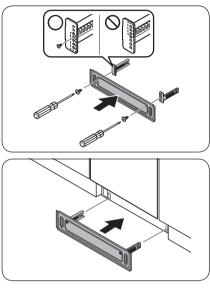
**2.** Attach the kickplate to the dishwasher using the kickplate brackets. Make sure the kickplate brackets are in the correct direction. See the figure for details.
