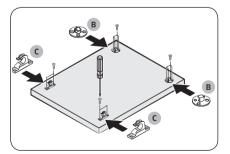
**4.** Remove the installation template and tighten the Custom panel fixers - Top (B) / Custom panel fixers - Bottom (C) at the top with 12 screws (C, Ø4 X 16) as shown.
