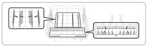
In the Upper rack, you can adjust the angle of the tines to two different positions to match the size and shape of your dishes. To adjust the tines, grasp the handle at the front of the rack, and then push it left or right. See the illustration below.
