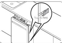
**2.** To prevent damage to the drain hose through the water supply line, slightly pull out the dishwasher and bend the built-in ear brackets of the left and right housings by 3/16" (5 mm). When done, reinsert the dishwasher with its center aligned.
