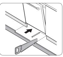
**3.** If you use the furniture plate instead of the kickplate, cut out the portion of the furniture plate that interrupts with the door before attaching the furniture plate to the dishwahser.
