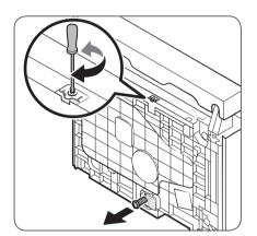
3. Turn the Torx T20 screwdriver counter clockwise as shown to remove the rear foot.
