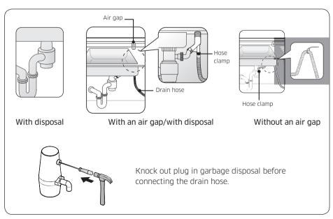
Drain system with a waste-disposal
