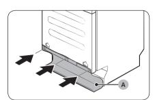
1. Insert the supplied rubber skirt (A) into the 3 holes at the bottom of the door.
