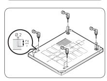
2. Put the installation template on the back of the custom panel and fix it temporarily using transparent tape. Note that the rear of the custom panel will be attached to the dishwasher door.
